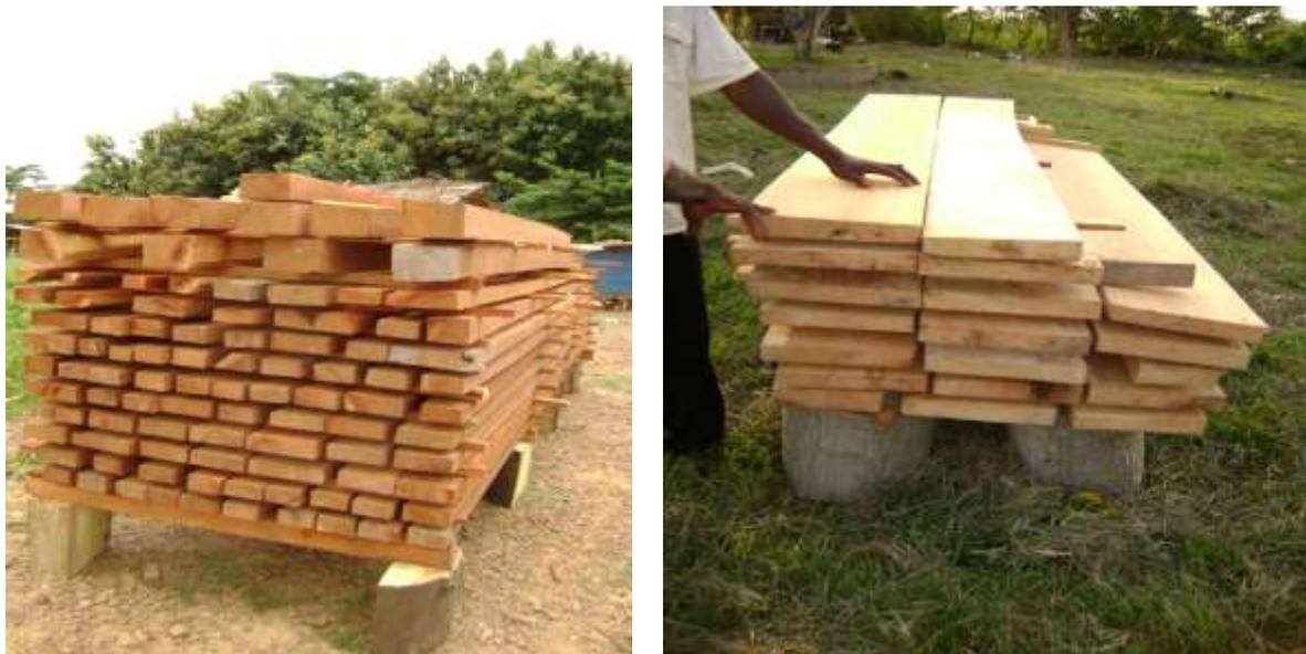
Figure 3: Stacked lumber produced with Logosol machine.
