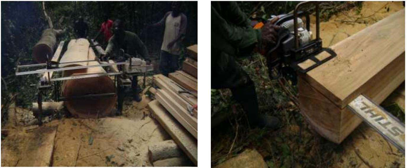
Figure1: Milling of logs using Logosol machines.
